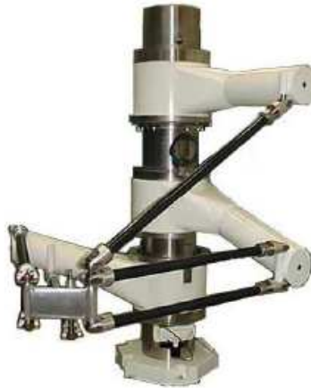
The ABB pick-and-place robot capable of performing two pick-and-place operations per second.
